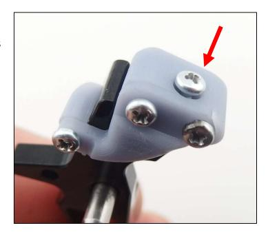
Make sure adapter will not hit sector gear teeth, otherwise grind the adapter to fit better on the trigger
